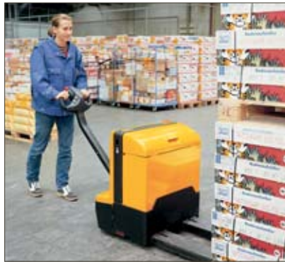
Collision protection on battery compartment
